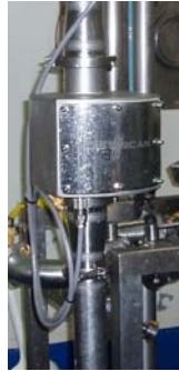
MA-700 In-pipe analyser immediately downstream of steam injection cooker
